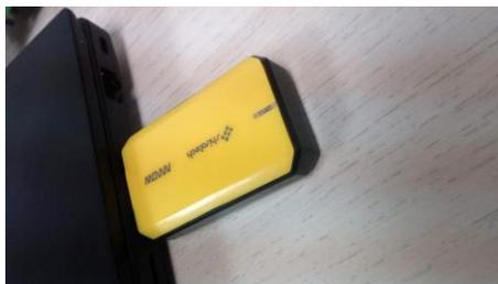
d. Turn on the iCOMOX by sliding the slide switch on the iCOMOX to the direction of the LED (the opposite direction of the USB-C cable).
