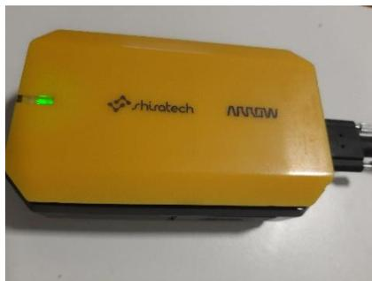
**Note, the iCOMOX is equipped with batteries. When the USB cable is disconnected, the iCOMOX, when turned on, is powered by the batteries instead of by the USB-C cable. Make sure that the iCOMOX is off when the USB-C cable is disconnected.**
